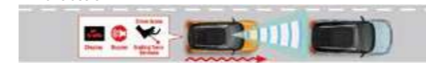
Deploys brake assist to increase braking force if the risk of collision is high and the driver panic brakes
